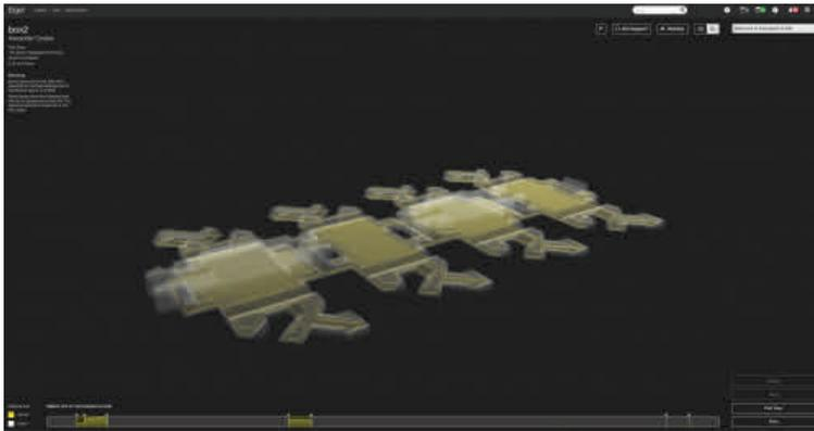
The full Eiger layout of the folding box. Sandwich panels strengthen each side of the box.
