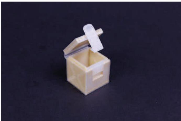
A box printed on the Mark Two with a living hinge for the lid and a flexural element for the latch.
