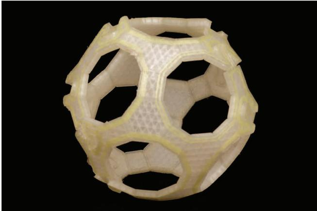
A polyhedron printed on the Mark Two with fiber-reinforced living hinges.
