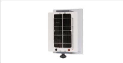
The 4-cell solar panel is used for experiments in photovoltaics and for generating electric energy for the electrolyzer. It can be turned in the frame for easier alignment to the light source.
